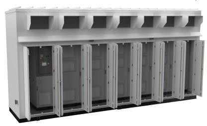
For the closed loop solution, depending on the drive rating and applicable heat-loss, one or two heat exchangers will be used. Heat exchangers can be attached to either end or at the back of the enclosure. If necessary, a motorized damper system on the partition barrier, and an electric heater will be included, supervised and controlled by the cooling system PLC. This allows the PowerFlex 6000 drive to provide pre-heating to the inlet air in cold conditions
