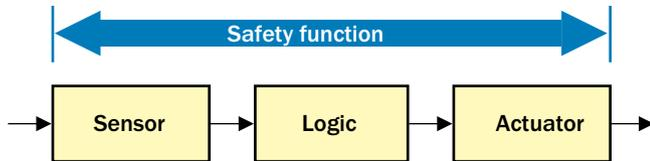
The actuator can involve several components (contactor, drive controller, feedback), depending on technical design and safety function. Braking systems and holding systems are also to be taken into account on axes subject to gravity.
