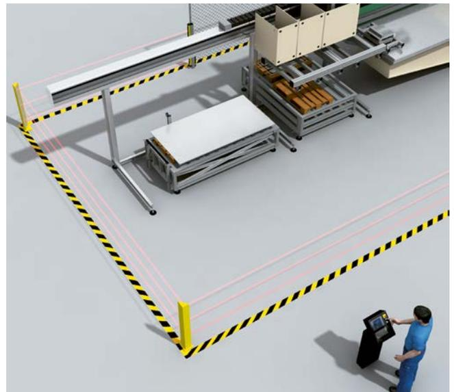
**Hazardous area protection: Detection of the presence of a person in the hazardous area**
