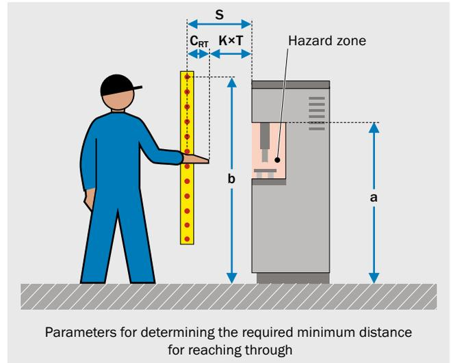
Parameters for determining the required minimum distance for reaching through
