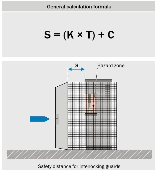
→ Calculation of the minimum distance for interlocking guards: ISO 13855 (B-type standard)
