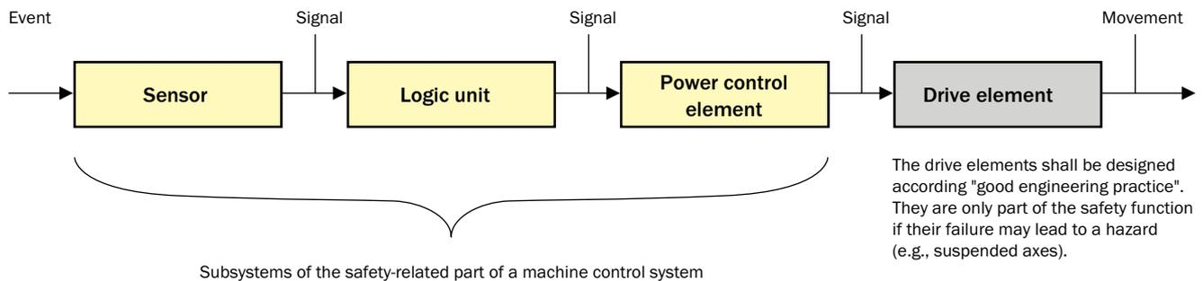
The drive elements shall be designed according "good engineering practice". They are only part of the safety function if their failure may lead to a hazard (e.g., suspended axes).
