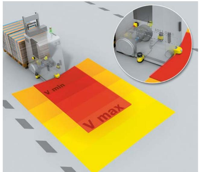
Speed monitoring for protective field switching on an automated guided vehicle
