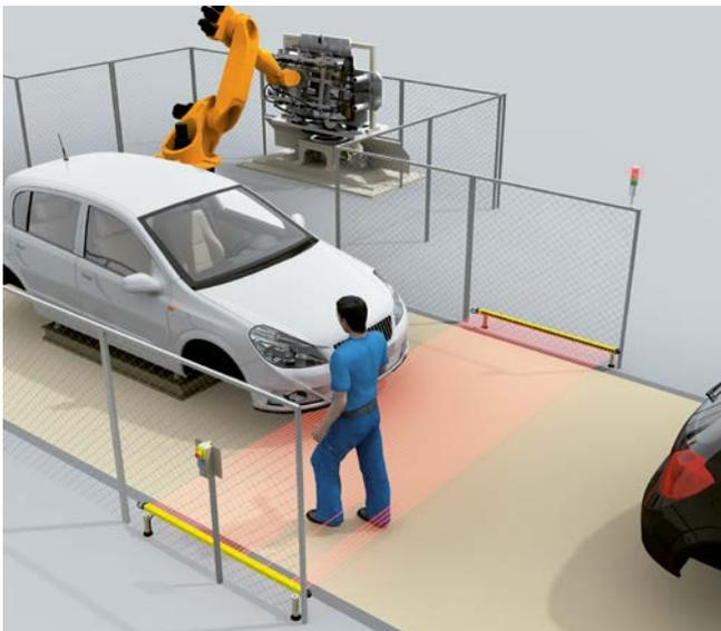
Entry/exit function with horizontally installed safety light curtain in a processing station on an automobile assembly line.
