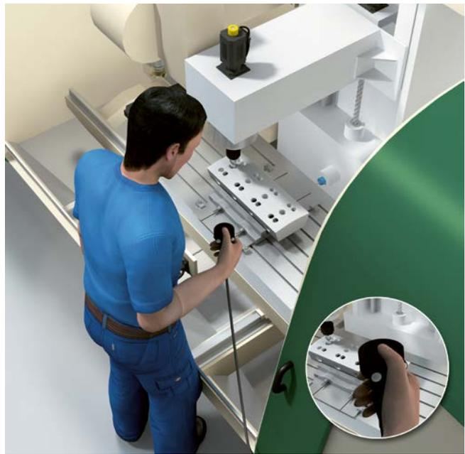
The machine start shall not be initiated solely by the actuation of an enabling device. Instead, movement is only permitted as long as the enabling device is actuated.
