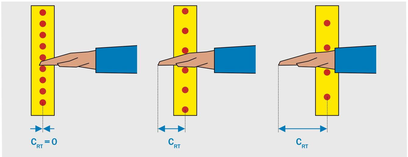
The figure shows an example of undetected depth penetration factor at safety light curtains with different detection capabilities.
