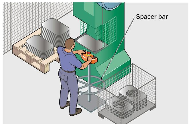
→ Requirements to be met by two-hand controls: ISO 13851 (B-type standard)
