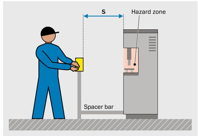
→ Calculation of the minimum distance: ISO 13855 (B-type standard)
