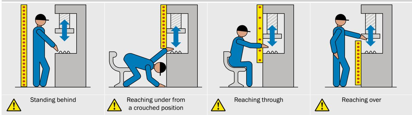
Once the minimum distance between protective field and the nearest hazardous point has been calculated, the protective field height required must be determined in a further step. This ensures the hazardous point cannot be reached by reaching over before the hazardous machine function has ceased.
