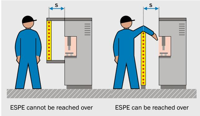
If access to the hazard zone by reaching over a protective field cannot be prevented, the height of the protective field and minimum distance of the ESPE must be determined. This is done by comparing the calculated values based on the possible detection of limbs or body parts with the values resulting from possibly reaching over the protective field. The higher value of this comparison shall be applied. This comparison is to be carried out according to ISO 13855, Section 6.5.
