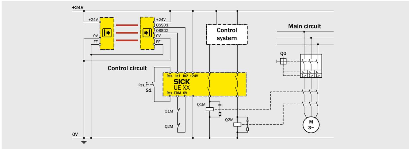
Safety relays combine one or more safety functions in one housing. They generally have automatic monitoring functions. The cut-off paths can be set up based on contact or using semiconductors. They can also have signaling contacts.
