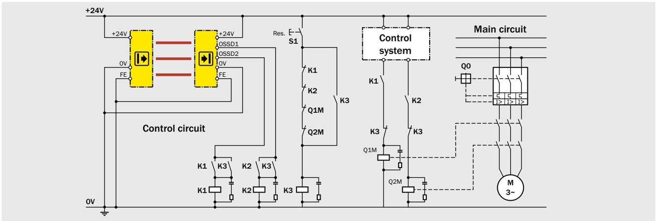
Using individual auxiliary contactors with positively guided contacts it is possible to design control systems with any level of complexity. Redundancy and monitoring by positively guided contacts are features of this safety principle. Wiring provides the logical operators.
