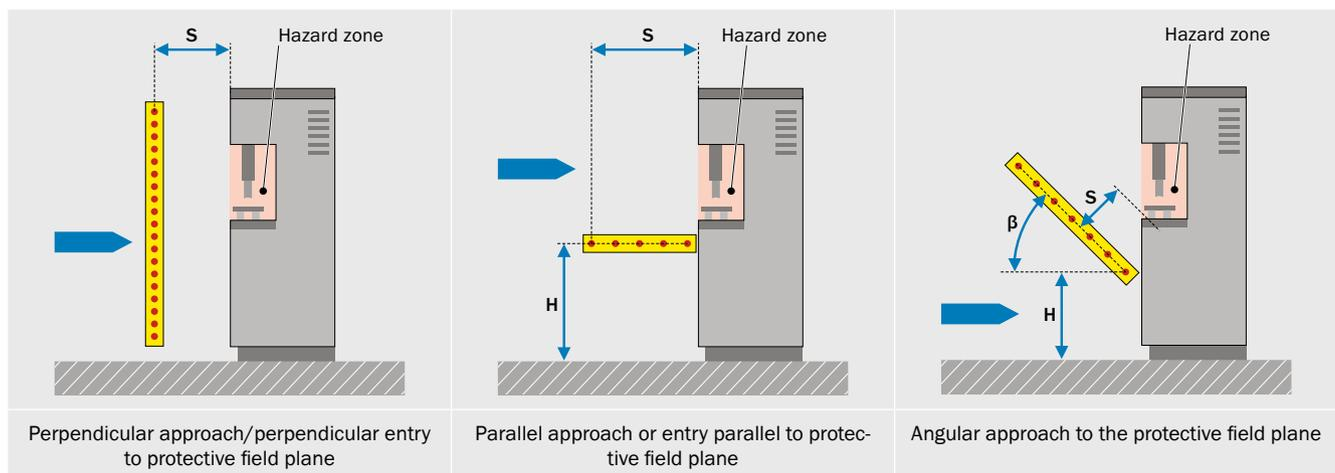
After the stop initiating ESPE has been selected, the required minimum distance between the ESPE's protective field and the nearest hazardous point is to be calculated.
