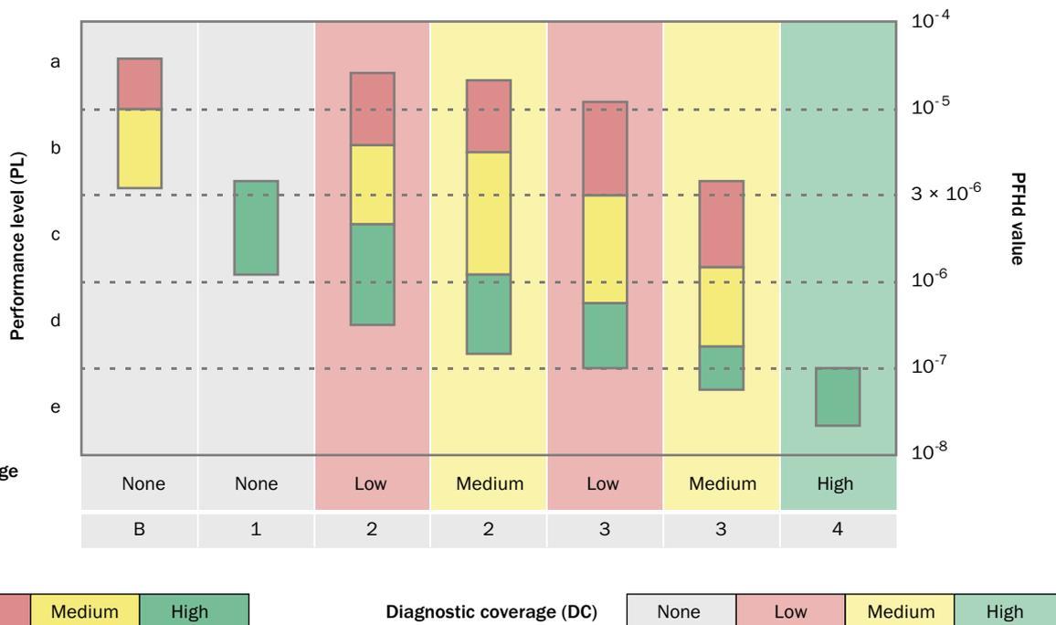
A performance level of "d" can be achieved with a dual-channel control system (category 3), for example. This can be reached either with components of good quality (MTTFd = medium) if almost all faults are detected (DC = medium) or with components of very good quality (MTTFd = high) if many faults are detected (DC = low).
