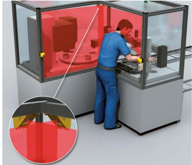
In this arrangement it is not possible to remain in the hazard zone without being detected. Therefore, a separate reset of the protective device is not necessary.
