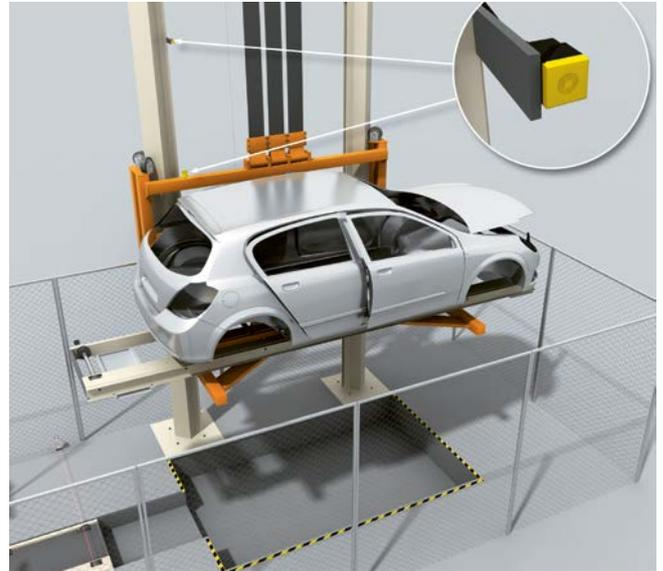
Safe position monitoring for a lift on an automobile production line
