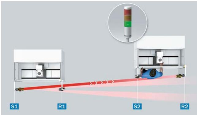
Mutual interference impedes detection by the ESPE and the hazardous movement is not stopped.
