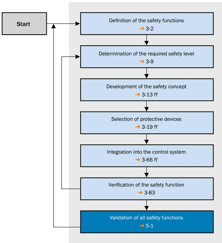
The purpose of the validation procedure is to check the specification and the conformity of how the components involved in the safety function have been integrated on the machine.
