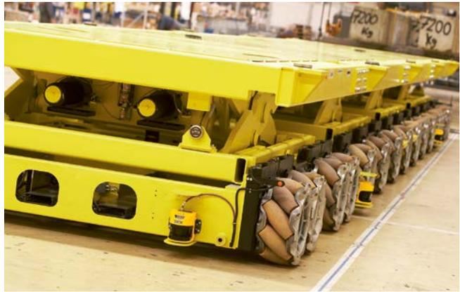
**Stationary application with an ESPE that moves with the tool**
