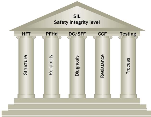
The safety integrity level achieved for a subsystem is made up of the following parameters:
