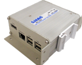
MC-2 Master Controller with up to 127 axis
